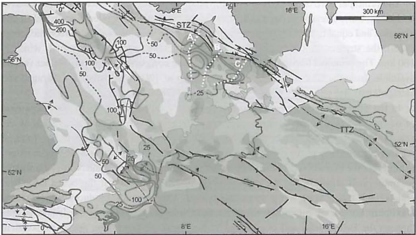
Figure 10.3 Inversion structures on the European continent (axes with anticline symbols) and the thickness of Late Cretaceous–Danian depocentres (yellow to brown colours increasing from 0–500 m, 500–1000 m, 1000–1500 m and >1500 m, respectively) and Middle–Late Paleocene depocentres (blue contours – labels in metres – with the red line indicating the depositional limit). The asymmetrical depocentres of the former are related to the primary, compressional, inversion and the more symmetrical and shallower Paleocene depocentres are related to secondary, relaxation, inversion. The depocentre east of the TTZ in Poland bounded by the green line represents Paleocene deposits <50 m. STZ is the Sorgenfrei–Tornquist Zone; TTZ is the Tornquist–Teisseyre Zone. The dotted white lines are the approximate locations of geological cross-sections (A, B, and C) shown in Figure 10.4. (The figure has been adapted from Nielsen et al. (2005).) For colour version, see Plates section.
